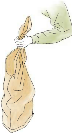
Figure 12A: Sandbag filled 1/4 to 1/3 full
